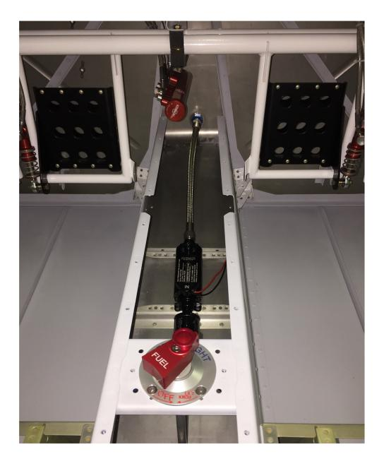
**Note-** The picture below shows the type 7 valve and the complex bend geometry to make the turn tight to the valve and yet clear everything and then make the bends through the tunnel out to the wings. Please note that with the wing root mounted filter setup, the rigid tube shown in this picture coming off of the bottom of the valve will be replaced with a flex hose.
