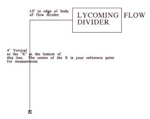
After building the correct template for either the AFP or Lycoming install, here is what you do with it. The measurement is taken off of the front of the Fuel Spider. The horizontal distances given are from the BODY of the spider. The vertical distance is from the center of the NPT port on the front of the fuel spider.
