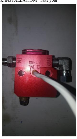
flow divider. Its orientation is aft, or perpendicular to the cross bolt holes in the body. This aligns with the flow divider fitting. Use a sharpie and place an index mark on the inboard edge of the transducer, Seal the NPT threads, tighten and orient the fitting to your index mark.
