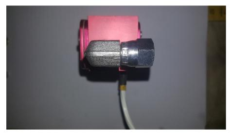
Remove the original 90\* adapter fitting from the flow divider, and replace it with the straight 1/8 NPT to -4 AN fitting supplied with the package. Seal the NPT threads, and tighten.
