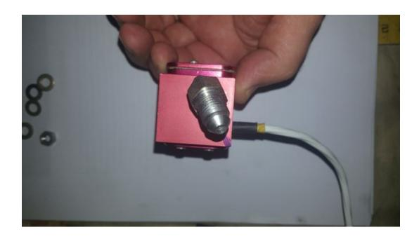
The outlet fitting is a 90\* ½ Male NPT to female -4 AN swivel fitting that connects the transducer to the flow divider. Its orientation is aft, or perpendicular to the cross bolt holes in the body. This aligns with the flow divider fitting. Use a sharpie and place an index mark on the inboard edge of the transducer, Seal the NPT threads, tighten and orient the fitting to your index mark.
