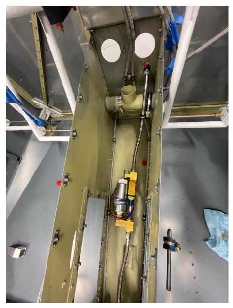
KIT 2 – This is installed exactly the same as kit 1 with the exception of the fact that the transducer no longer is mounted in the tunnel. So you will go directly from the fuel pump to the firewall. (Image at left shows the forward section of kit 2. This is also the image with wing root filters which is why there is no filter in the tunnel. If you are using kit 2, you will still have your filter in the tunnel aft of the firewall just like kit 1.
