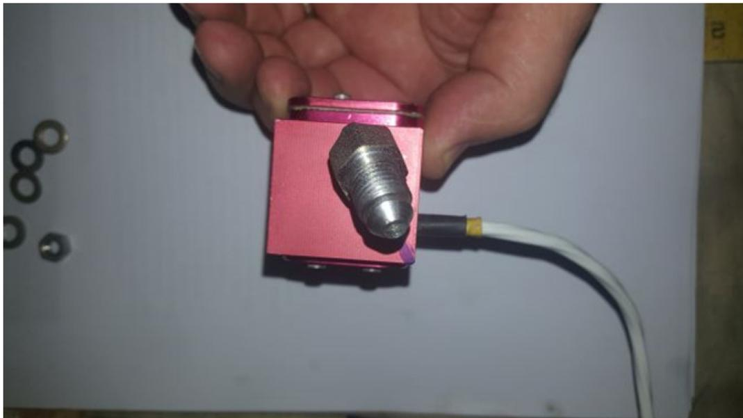
The outlet fitting is a 90° 1/4 Male NPT to female -4 AN swivel fitting that connects the transducer to the flow divider. Its orientation is aft, or perpendicular to the cross bolt holes in the body. This aligns with the flow divider fitting. Use a sharpie and place an index mark on the inboard edge of the transducer, Seal the NPT threads, tighten and orient the fitting to your index mark.
